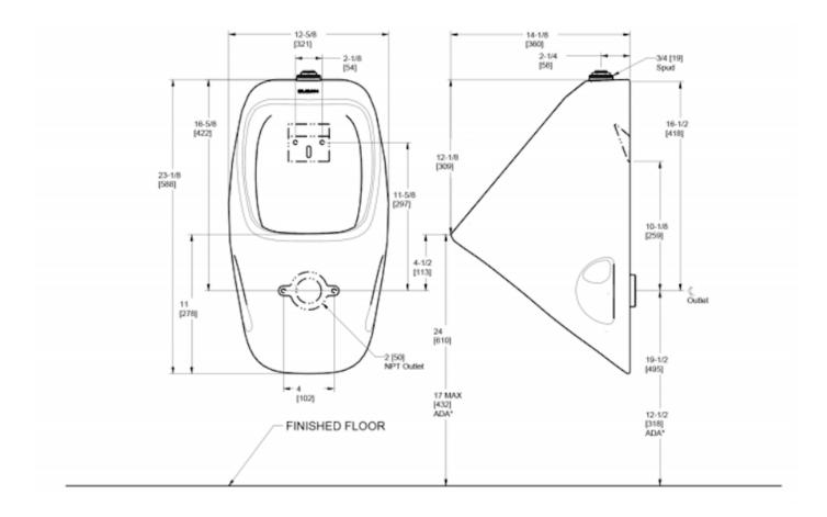
NOTE: ADA urinal rim height requirements allow all heights 17" and below. Sloan strongly recommends roughing in the drain to achieve a 16<sup>1</sup>/<sub>2</sub>" rim height or less to ensure compliance.
