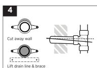
**ADJUST DRAIN TO ACHIEVE PITCH** If standing water is present (code requires 1/4" drop per foot of drain line for proper pitch). Seal wall according to code.
