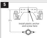
MEASURE & MARK THE ROUGH-IN If in-wall carrier is not used. Use a 5/16" masonry bit to drill hole, then install the hanger bracket with one plastic anchor and screw
