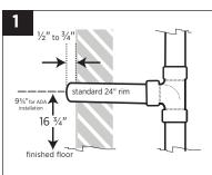
SET DRAIN HEIGHT 16 3/4" from finished floor (standard 24" rim) or 9 3/4" for ADA installation. Threaded nipple should extend 1/2 to 3/4" from wall.
