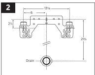
**CARRIER STUD PLACEMENT** If using in-wall carrier, set bearing as shown above.
