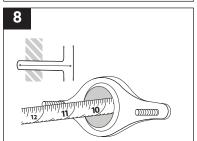
**DETERMINE THE DRAIN NIPPLE DEPTH** by measuring the distance between the back of the sanitary tee (or elbow) to the front edge of the elagin.
