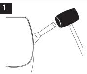
USE UTILITY KNIFE TO CUT CAULK then use a putty knife and mallet to remove the bowl. Remove hanger brackets, scrape off caulk, and clean the wall.
