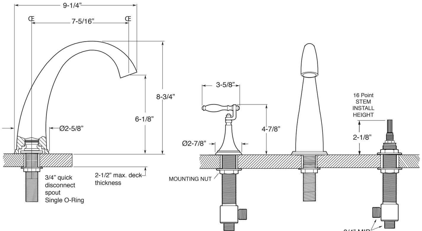
Spout and valves install through 1-1/4" diameter holes.
