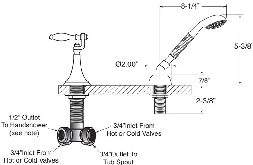
NOTE: 1/2" outlet for in-line vacuum breaker (18.15.055), and 60" chrome spiral hose (18.10.016) - INCLUDED
