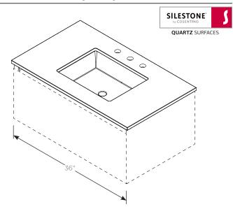
Note: Sinks must be located over H1-Tip Out or H2/V14 Plumbing drawers. See Cartesian Reference Guide for more information.
