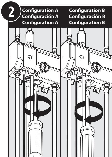
Loosen Filter Plug with flathead screwdriver.
