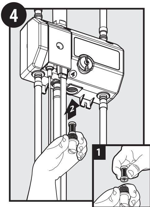
Firmly push new Filter onto New Filter Plug and re-insert Filter Plug into Control Box.
