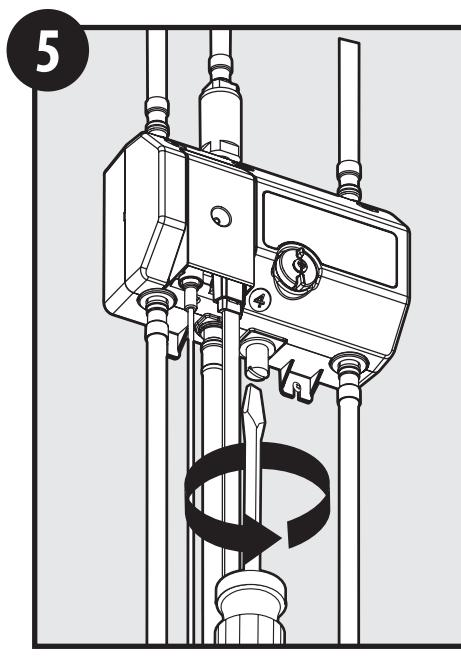
Tighten Filter Plug with flathead screwdriver.
