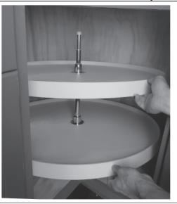
Insert one Shelf Hub through the bottom of a shelf as shown. Place one Shelf Hub Cone on the top of the shelf and fasten using (3)  $\#8 \times 1/2$ " Flat Head Machine Screws provided. NOTE: Make sure the rib inside the Shelf Hub Cone is aligned with the groove in the hub (see picture). Repeat with second shelf.
