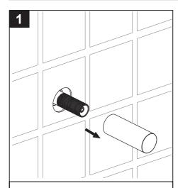
Turn the water off. Remove the mud guard.
