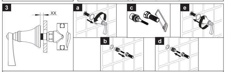
Note the measurement between the finished wall and the bottom of the escutcheon.
