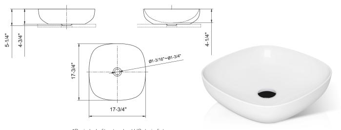
\*Drain hole fits standard US drain fixtures
