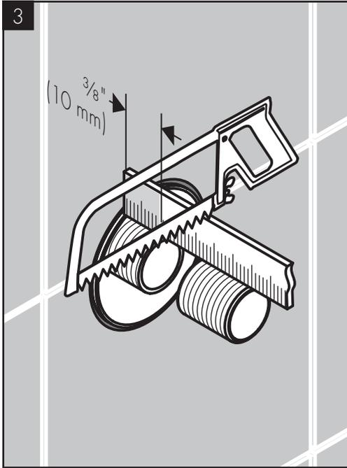
Cut the slip connector so that they extend  $\frac{3}{8}$ " (10 mm) outside the surface of the finished wall.
