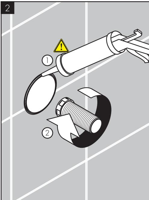
Seal the wall around the plaster shield using water-proof sealant.
