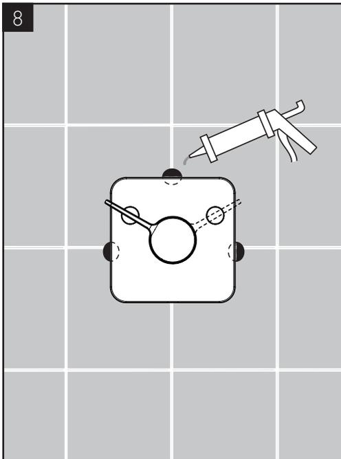
Place a dab of waterproof sealant on the wall at the grout joints.
